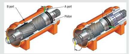
Cutaway on left shows initial positions of piston (green line) and output shaft. (yellow line). Pressurized fluid entering the inlet port pushes on the piston; a stationary ring gear causes the piston to rotate clockwise. At right, teeth on the output shaft mesh with those on in the ID of the piston, causing the shaft to rotate clockwise relative to the piston. Pressuring the B port returns the piston and shaft to their in initial positions.
