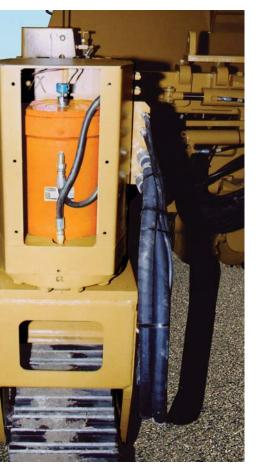
Even if Helac's L-30 series rotary actuator didn't provide a simpler, more compact design than conventional steering cylinder assemblies, its steering angle is more than twice that of cylinders — still making it an attractive alternative.
