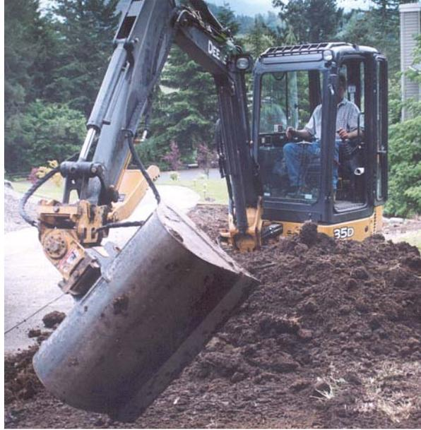
PowerTilt is specifically engineered to work with a variety of attachments, improving your machine's versatility. PowerTilt is compatible with wide buckets, brushcutters, narrow buckets, hydraulic hammers, rippers and mowers — just to name a few.
