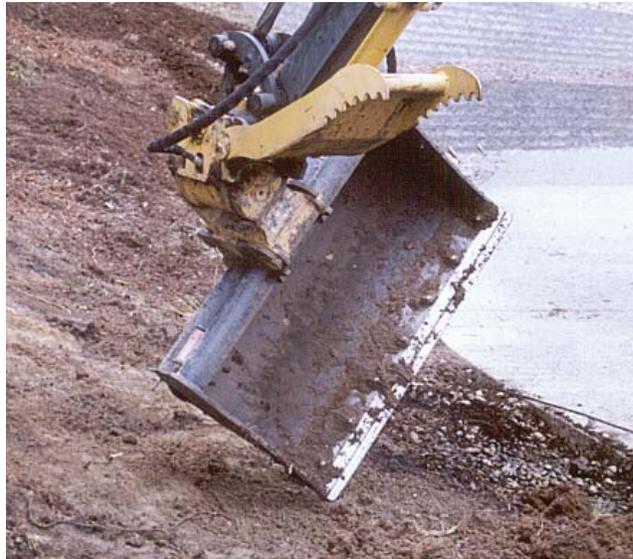
any more than absolutely necessary. “Our PowerTilt provided us with the ability to position the attachment instead of the machine,” Magstadt explained. “In landscaping construction, I’m in a lot of tight areas. With
