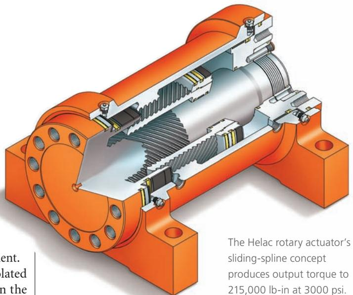
The Helac rotary actuator's sliding-spline concept produces output torque to 215,000 lb-in at 3000 psi.
